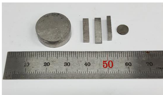
Figure 2. Typical dense pellet of bulk KBT by SPS with a typical diameter of 18 mm and a thickness of \sim 6 mm to 7 mm (left) and specimens cut for measuring electrical (bars, middle) and thermal transport properties (disk, right).
